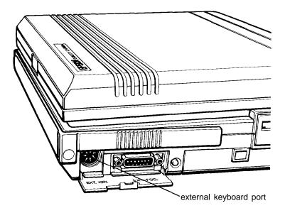
3. Attach the keyboard adapter to the external keyboard slot. Then attach the connector from the external keyboard to the adapter.
